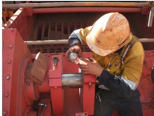
Photo No 29: Top Excitor Counter Weight being re-orientated
