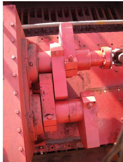
Photos No 14 and 15: Original and re-oriented position of counter weights on actuator.
