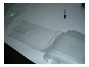
Open the sample into a flat sheet and mark off the required test points at 240mm and 120mm centers, allowing for at least 5 test points of the base material, and 5 test points of that part of the material which has been folded or creased.
