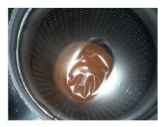
If the material has not broken through as shown in the above photo, the dart impact value is greater than 50 grams. Add additional weight to the dart, move the material to a new test point and repeat the test, continuing the process until the dart breaks the material, but does not pass straight through the material.
