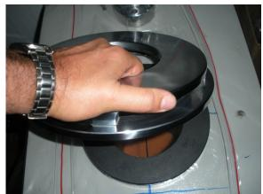
Fit the 50 gram dart into dart clamping unit.
