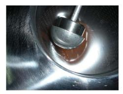
Verify the impact load by performing several tests at the same dart load
