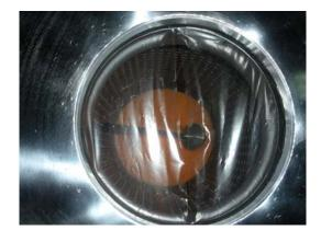
Once the seam impact load has been determined and verified, mount the material sample so that the dart impact point is on the base material.
