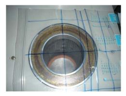
Perform the same sequence of tests, adding additional weight to dart until it breaks through the material as described previously.
