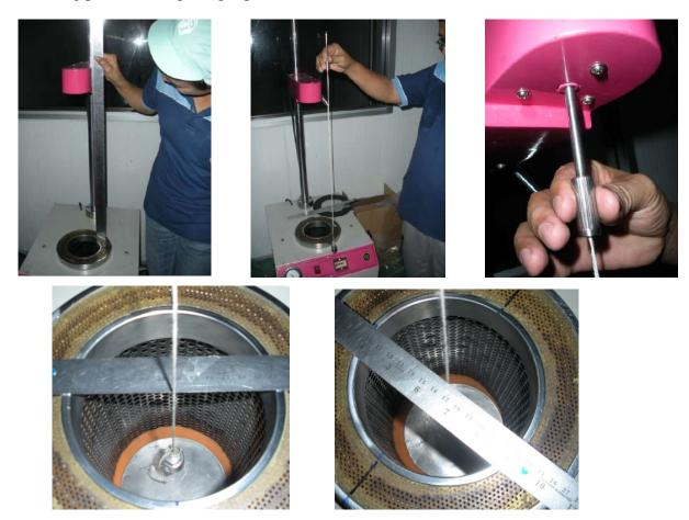
The plum bob needs to be suspended from the centre of the dart clamping unit, using the manufacturer's spigot. The height of the cross head initially needs to be referenced at 600mm from the top of the sample mounting plate for performing comparative tests, and in accordance with ASTM D4272 - 09 for performing absolute tests. Remove the plumb line on completion.
